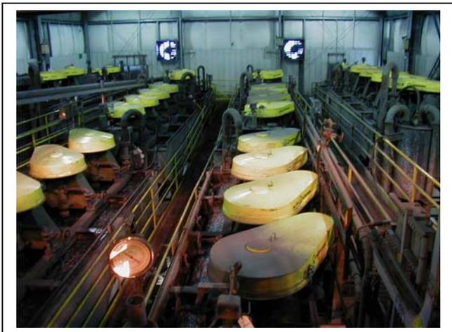
Zinc and lead flotation cells in Greens Creeks new cleaner flotation plant. Greens Creek Mine, Admiralty Island, Alaska.
